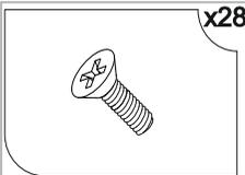
x28<br>Винт М6х20 |
